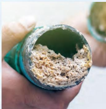
The Water Reclamation Facility receives and treats approximately 10,000 pounds of food-grade fats, oils, and grease (or "FOG" in industry jargon) every day. These substances are difficult and costly to treat. FOG can cause sewer backups in your pipes that are costly and inconvenient to remove. In fact, grease is one of the leading causes of sewer clogs and overflows.
